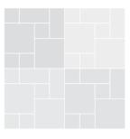
Note: The repeating modular pattern shown can be created using the contents of a single box of the 1000x1000mm Modular Panel listed below. Each box cotains the following sizes: 500x500mm (x2), 500x250mm (x2) and 250x250mm (x4), it can then be reapeated to cover the installation area, as shown above.
